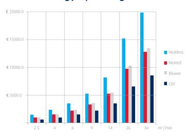
Data assumes nominal conditions, 6000 operating hours per year, 0.12€/kWh utility rate, compressor generation efficiency of 5.5 kW/m³/min
