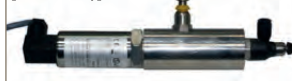
Hygrometer sensor in partial flow bypass tube
