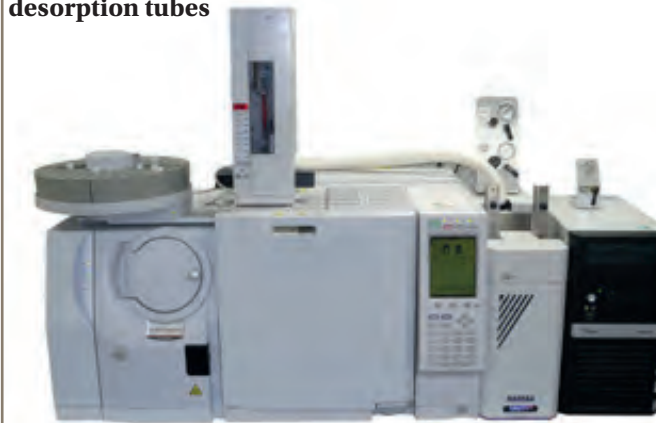
Example of Gas Chromatograph (GC) required to analyse oil vapour samples collected in the thermal desorption tubes
