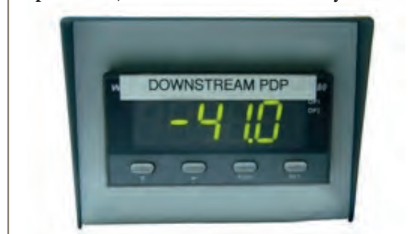
Example of a typical hygrometer using electrical sensing method based upon capacitance, resistance or conductivity
